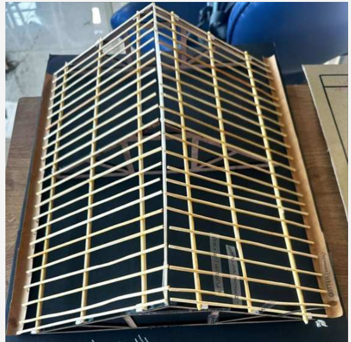
Scaled model of a wooden truss in an Integrated workshop on skills with building technology, enhancing their understanding of wooden joinery and roof truss.
